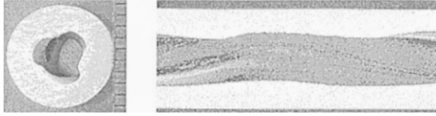
Figure 1: Radial and axial cross-sections of the stamped membrane [1].
